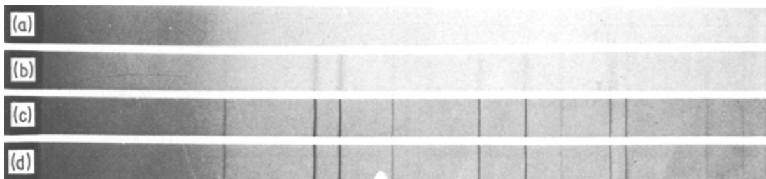
Figure 1 X-ray diffraction patterns of (a) ferric oxide hydrate dried at 100°C, (b) \alpha -Fe 2 O 3 obtained from the ferric oxide hydrate (350°C, 4 h), (c) \alpha -Fe 2 O 3 obtained from the ferric oxide hydrate (900°C, 2 h), (d) pure commercial iron (III) oxide.
